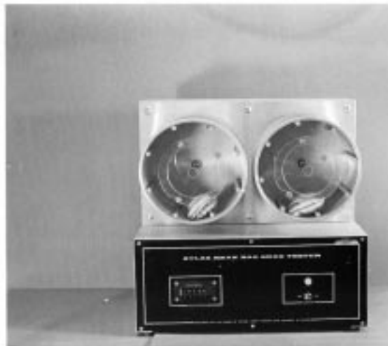
FIG. 4 The Bean Bag Snag Tester With Two Test Chambers
