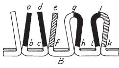
ad = cut pile tuft element gj = loop pile tuft element ab, cd, ef, gh, ji, jk = tuft legs cd, ef = cut pile tuft leg pair ij, jk = loop pile tuft leg pair, a loop B = one binding site
