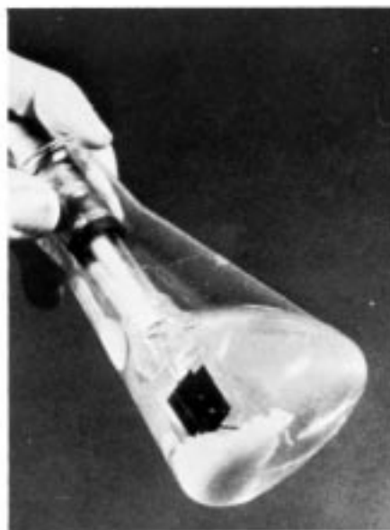
FIG. 2 Dip Cell Immersed in Flask
