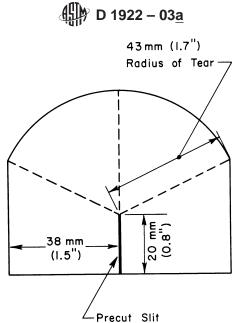
FIG. 1 Constant-Radius Test Specimen for Tear Resistance Test
