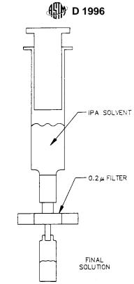
FIG. X1.2 Final Preparation of Sample Extract
