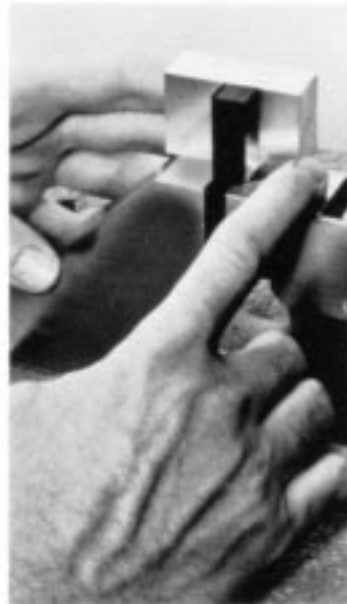
FIG. 4 Jig for Positioning Specimen for Clamping
