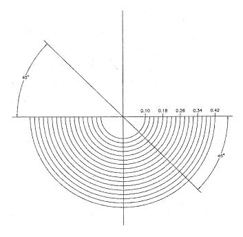
$\label{eq:Note_loss} Note \ 1 \\ \hline \textbf{--Magnification} = 100X.$  FIG. X1.2 Example of Transparent Template for Determining Radius of Notch
