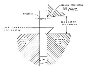
PLANES C AND D MUST BE PARALLEL TO WITHIN 0.025 MM (0.001 IN.) OVER A DISTANCE OF 25 MM (1 IN.)
