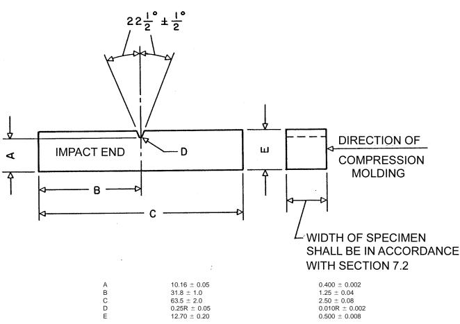
FIG. 6 Dimensions of Izod-Type Test Specimen
