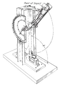
FIG. 3 Cantilever Beam (Izod-Type) Impact Machine
