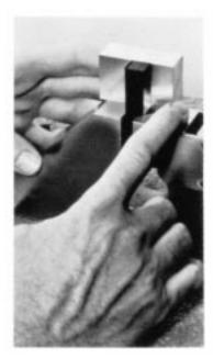
FIG. 4 Jig for Positioning Specimen for Clamping
