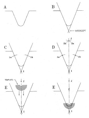
FIG. X1.4 Determination of Notching Radius
