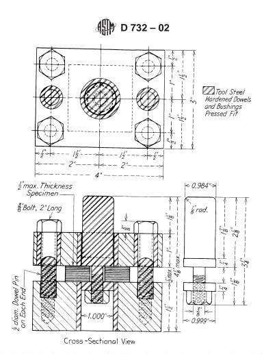
Note 1—In case of difficulty in obtaining hardened dowels and bushings, the entire shear tool may be made from a fairly good grade of steel, eliminating all of the bushings shown. The actual working surfaces will wear faster than when hardened tool steel is used. When they show signs of appreciable wear, the shear tool can then be bored out to take either hardened or unhardened bushings, depending upon which are available.
