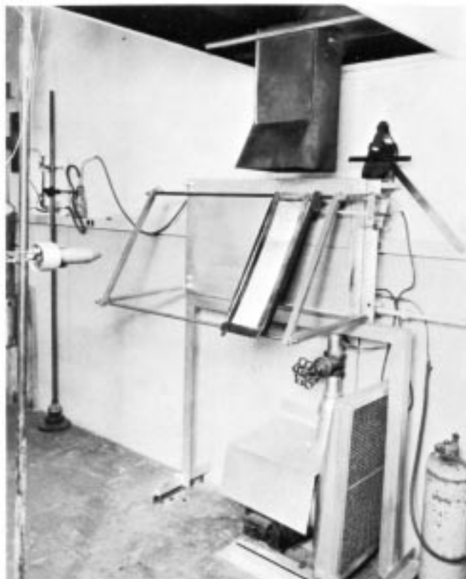
FIG. 1 Radiant Panel Flame Spread Test Equipment
