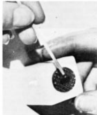
FIG. 3 Embedding Rubber Block in Mucilage
