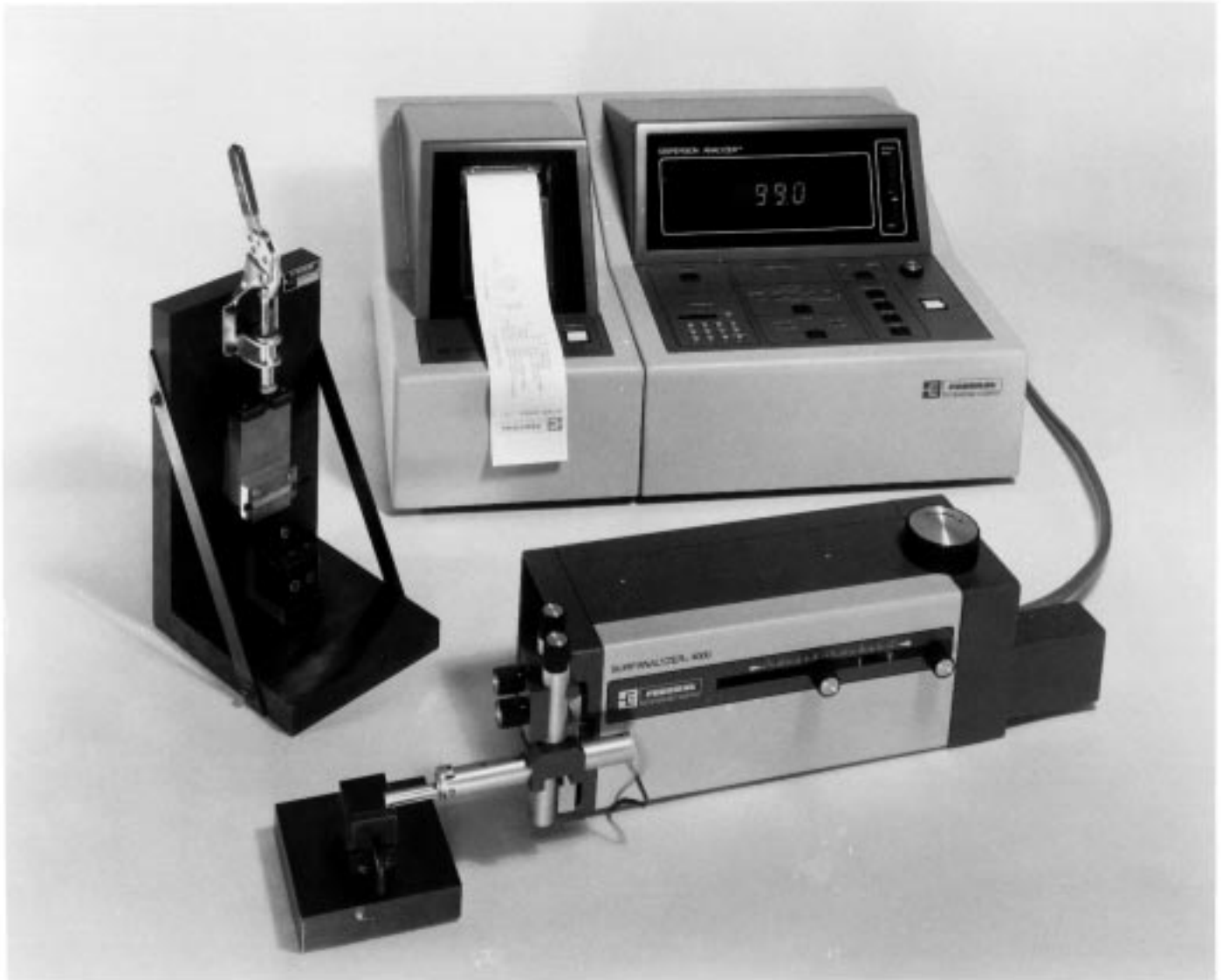
FIG. 6 Components of Dispersion Analyzer System
