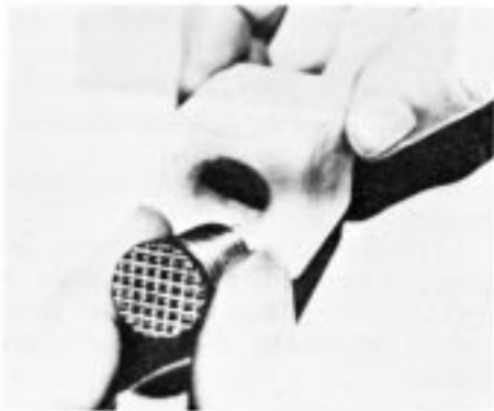
FIG. 2 Brass Sample Mount and TFE-Fluorocarbon Insulator
