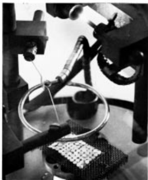
(c) Evaporation of Carbon on to Poly (Vinyl Formal) Coated Grids
