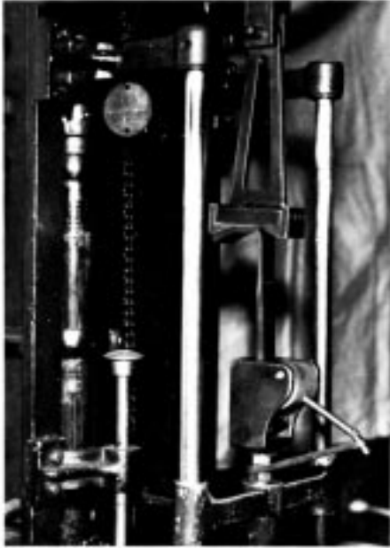
FIG. 5 Adhesion Tensile Testing Fixture in Operation
