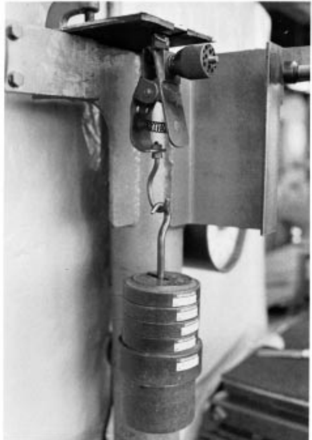
FIG. 12 Test Apparatus For Static Mass Adhesion Test on Rubber Tank Lining
