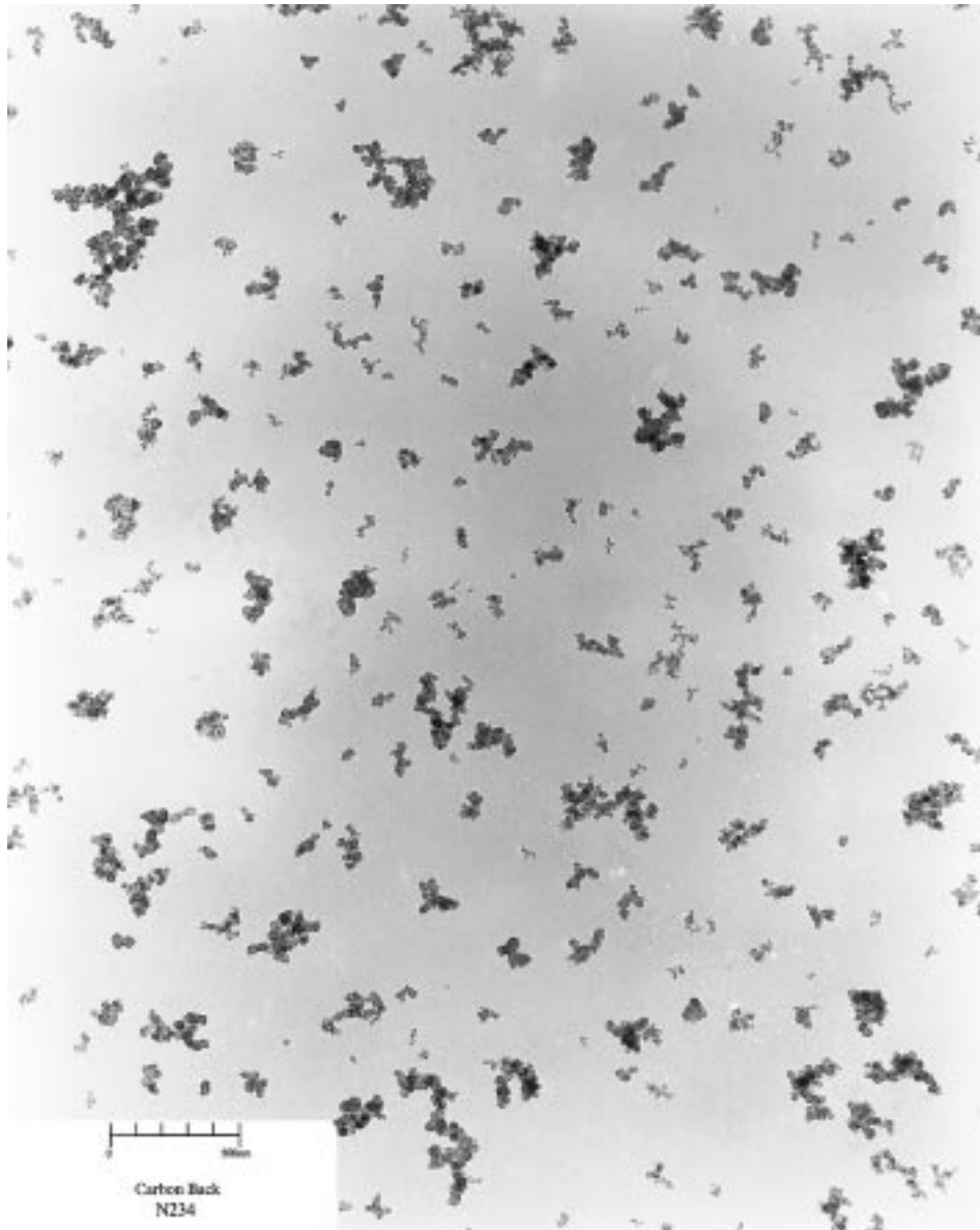
FIG. A1.9 N234 Carbon Black, Scale = 500 nm
