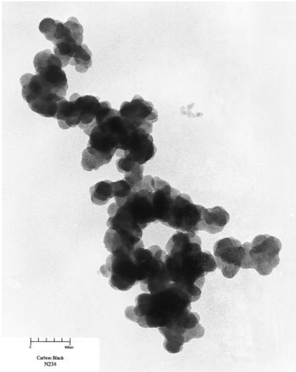
FIG. A1.10 N234 Carbon Black, Scale = 50 nm
