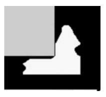
Note 1—Fig. A1.3 illustrates the condition of a sharp edge meeting the requirements of Test Method D 877. Note the sharp edge fits into the radius gage and only one side of the gage fits up against the disk while the other side has considerable space.
