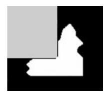
Note 1—Fig. A1.2 illustrates the case where the edge has a radius equal to the gage. Note both edges fit to the edge of the gage and the disk edge fits in the radius with no gap as in Fig. A1.1. This disk is acceptable, however, consideration should be given to machining the disk to a sharp edge because any degradation will make it unacceptable.
