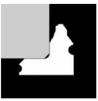
Note 1—Fig. A1.1 illustrates the case where the edge radius of the disk exceeds the allowable radius. Both sides of the gage are flush with the disk, and the edge of the disk does not fit into the gage. This condition requires that the disk be machined back to a sharp edge. See Fig. A1.3 for a sharp edge.
