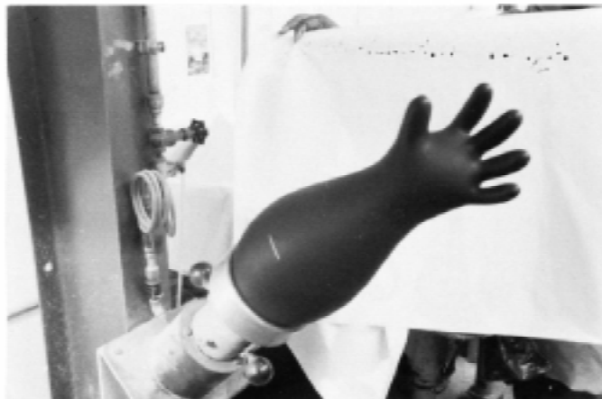
NOTE—Glove inflated to maximum allowable degree. FIG. 37 Inflator (Glove Inflated to Maximum Allowable Degree)
