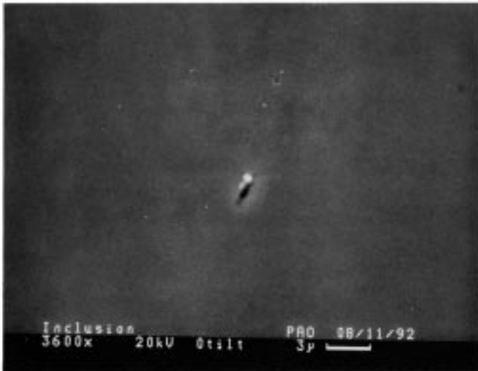
FIG. 2 Example of Pit Defect (3600 × magnification)
