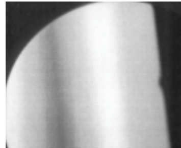
FIG. 41 Dimples Under Fluorescent Lighting Conditions Distort the Reflected Image.
