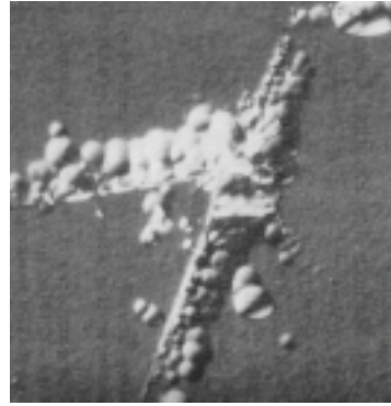
FIG. 33 Crack, Resulting from the Impact on the Wafer Surface, Following Preferential Etch, Magnification 450 \times .
