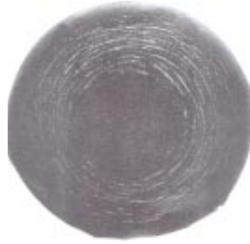
FIG. 27 A-swirl on as Grown Float-Zone Silicon Following Preferential Etch, Full Wafer View.
