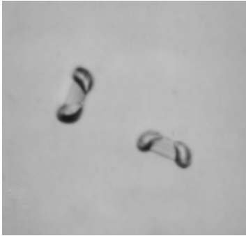
FIG. 12 Oxidation Induced Stacking Faults on (100) Silicon Following Oxidation and 4-min Wright Etch, Magnification 200 \times .
