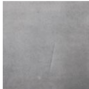
FIG. 53 Groove or Micro-Scratch, Magnification 220 \times .
