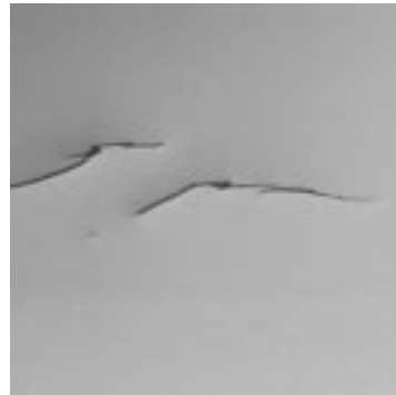
FIG. 35 Crack on a Wafer Surface Due to Mechanical Contact, No Preparation Required, Magnification 750 \times .
