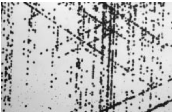
FIG. 23 Copper-3 Etch Without Agitation, Slip Dislocations, 100x, p type, 10 ohm-cm, [111], 10 μm removal.
