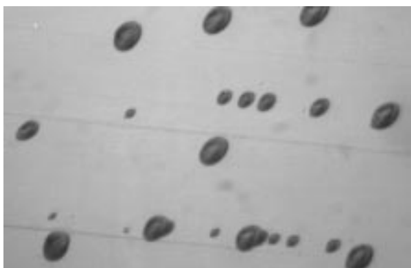
FIG. 22 Copper-3 Etch Without Agitation, Dislocations, 500x, p type, 10 ohm-cm, [100], 10 μm removal.
