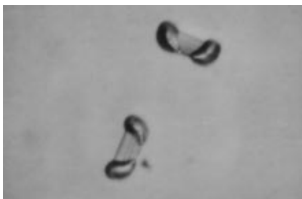
FIG. 20 Copper-3 Etch Without Agitation, Oxidation Stacking Fault, 1000x, p type, 10 ohm-cm, [100], (1100°C Steam, 80 minutes), 1 μm removal.
