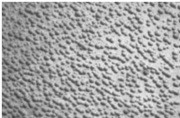
FIG. 18 Copper-3 Etch With Agitation, Shallow Pits (Haze), 500x, p type, 10 ohm-cm, [111], (1100°C Steam, 80 minutes), 2 μm removal
