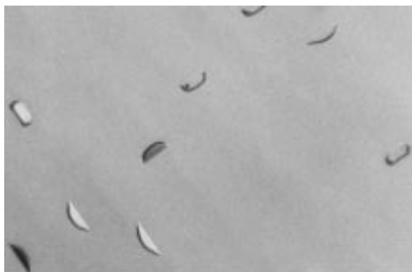
FIG. 8 Wright Etch With Agitation, Bulk Oxidation Stacking Fault, 500x, [100], (1100°C Steam, 80 minutes).
