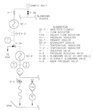
Note 1—Fixed back pressure regulating valves (V4) are available and eliminate the need to adjust back pressure and readjust the flow. This fixed pressure regulating valve provides the added benefits of acting as a sample relief valve and grab sample discharge.
