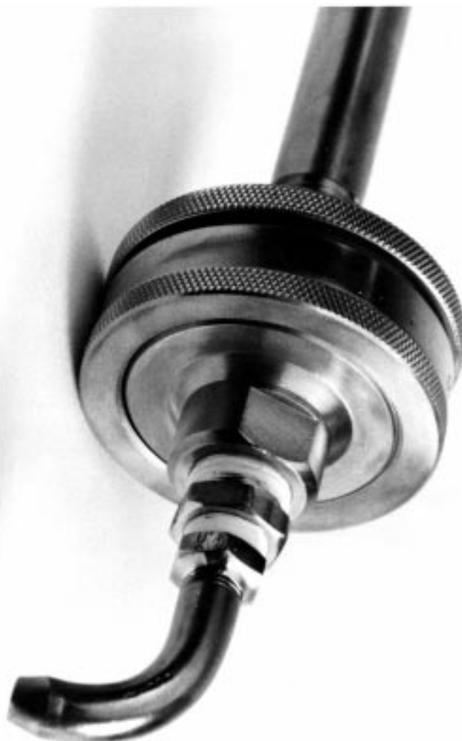
FIG. 6 Typical Holder for Flat, Round Filters
