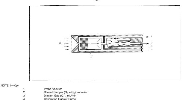
$\label{eq:Q2} \mbox{Gas being sampled, mL/min} \\ \mbox{NOTE 2-Dilution Ratio} = Q_2/(Q_1 + Q_2).$
