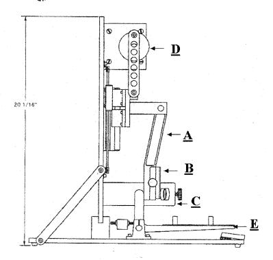
NOTE 4—Legend: A—motor-driven balanced arm B—cutting edge C—mandrel D—motor/drive wheel E—weights
