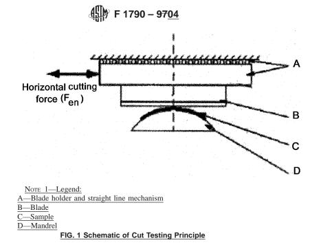
6.2 *Mandrel*—The top surface of the mandrel is a rounded form which has an arc of <u>at least</u> 32 mm-([1.25 in.)] in a circle having a radius of 38 mm-([1.5 in.)]. The surface of the mandrel should either be made of electroconductive material or be covered with an electroconductive material. Double-faced tape is used to secure the specimens to the electroconductive surface. material.
