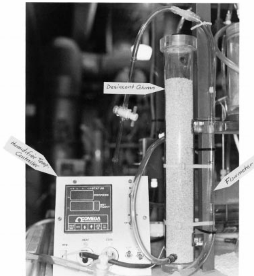
FIG. 3 Detail of Desiccant Column and Flowmeter
