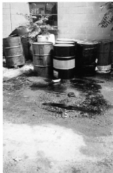
FIG. X2.12 Surface Staining from Improper Drum Storage
