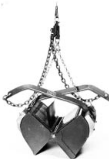
FIG. A1.5 Van Veen Grab (Photograph courtesy of Kahl Scientific Instrument Corp.)
