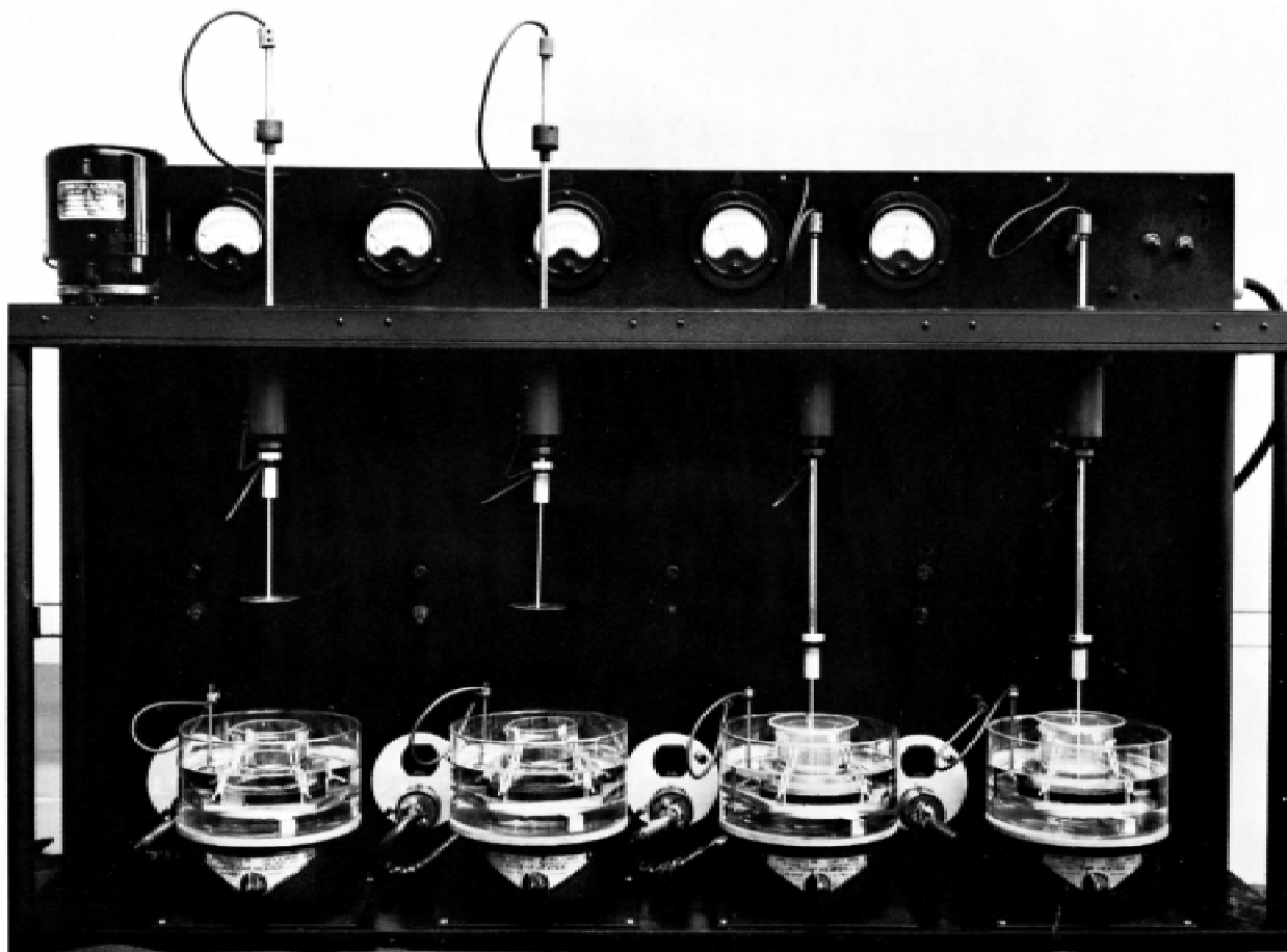
FIG. 12 Multiple-Cell Electroplating Apparatus
