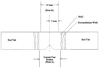
Note A—No plastic deformation from previous testing is permitted in the region between the HAZs caused by the reconstitution welds (the central test section). Note B—Temperature during welding shall not exceed the irradiation temperature.
