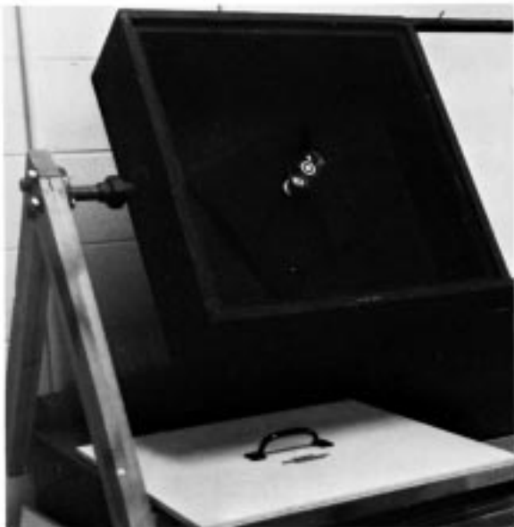
FIG. 1 Typical Unit with Pyranometer Mounted in Black Box
