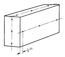
Note 1—The dots on the center line of each face are  $\frac{1}{2}$  in. (13 mm) in from each edge, and the cross on the axis is in the center. These positions indicate the points at which three measurements for each dimensions are to be made.
