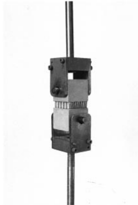
FIG. 1 Flatwise Tension Test Setup
