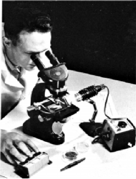
FIG. 1 Suitable Microscope: Inclined Binocular Body; Mechanical Stage; Triple Nosepiece; Ocular-Objective Combination to Obtain 40 to 45× and 90 to 150× Magnification
