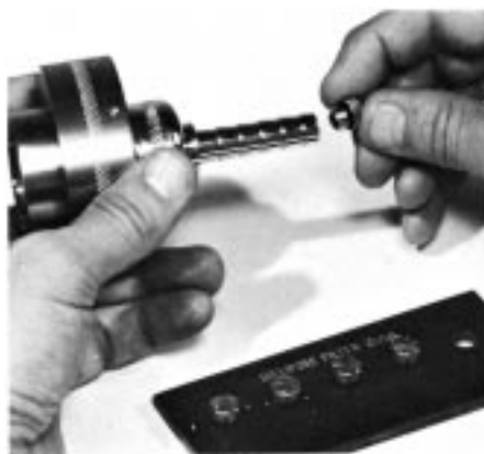
FIG. 5 Inserting a Typical Orifice
