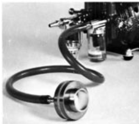
FIG. 3 Typical Air-Sampling Filtration Apparatus
