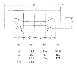
Note—The cutting edges shall be beveled on the outside and straight on the inside. The die shall be kept sharp and free of nicks to give clean, even edges on the specimen.
