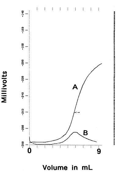
$\frac{\underline{A}}{\underline{B}} = \frac{\underline{titration \ curve}}{\underline{first \ derivative \ curve \ of \ Curve \ A}}$
