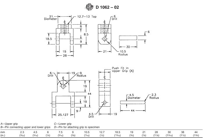
FIG. 1 Details of Test Grips
