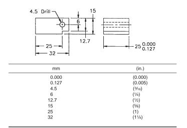
Note 1—The 1-in. (25-mm) square surface to be glued shall be ground flat and parallel with the opposite surface.
