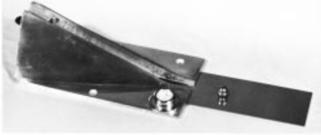
FIG. 1 Adhesion Test Apparatus and Specimen Showing Distance of Roll That is Measured
