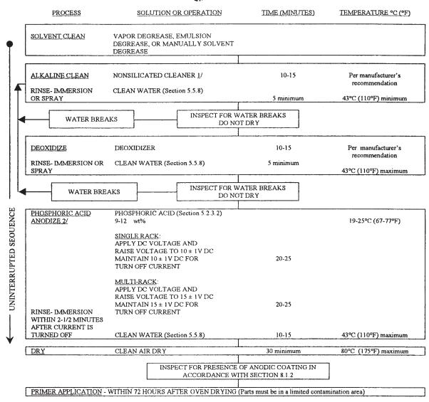
NOTE 1—Experience has proved nonsilicated cleaners to be preferable when reprocessing might be involved. NOTE 2—A single-rack facility is one with a single anode rack between each set of cathodes. A multi-rack has two or three anode racks between each set of cathodes.
