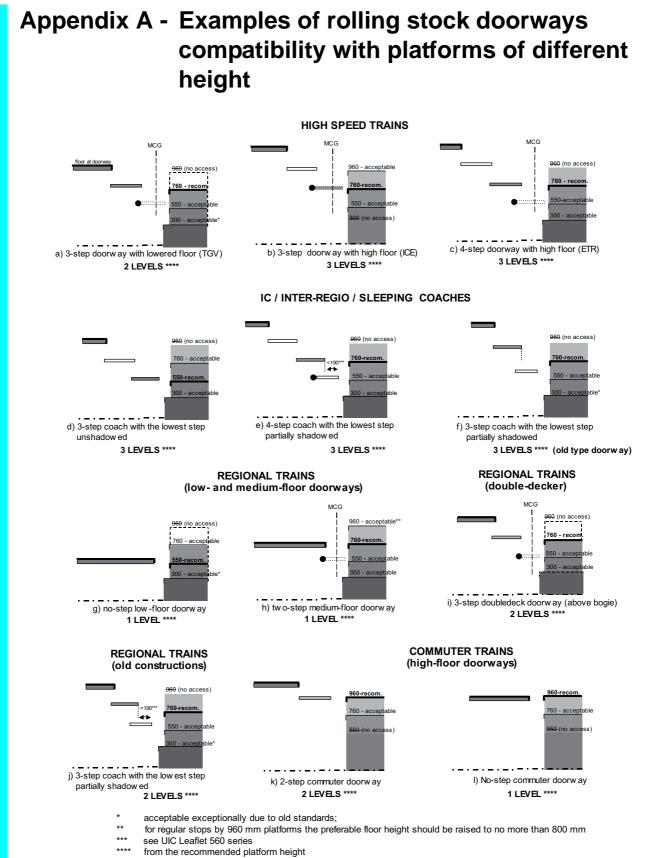
MCG maximal construction gauge acc. to UIC Leaflet 505 series
