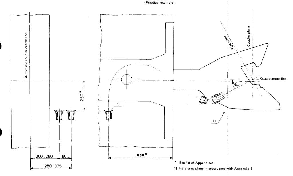
POSITION OF THE JUNCTION BOX ON THE HEAD STOCK OF WAGONS WITH TYPE 2 UIC/OSJD SUSPENSION (TELESCOPIC-LEG SUSPENSION)
