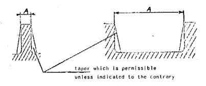
The tolerances apply to the dimension A neglecting the taper.
