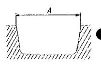
The tolerances apply to the dimension A, measured at the point where the dimension is indicated.
