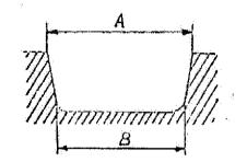
The tolerances apply to the dimensions A and 8 (the value of one of them can be calculated, where applicable, from the taper indicated on the drawing):
