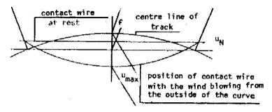
Residual bow width w.: Horizontal distance between the contact wire and the end of the bow.
