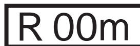
Fig. 1 - Sign for the radius of the smallest curve that the design of wagon can negotiate
