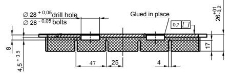
Design and measurements of the grooves should only be considered as examples
