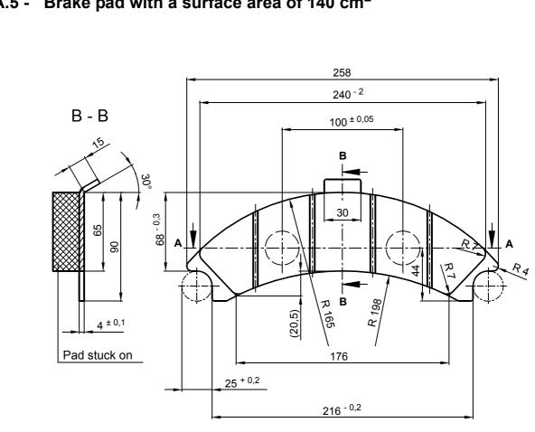
Brake pad with a surface area of 140  $\text{cm}^2$ A.5 -
