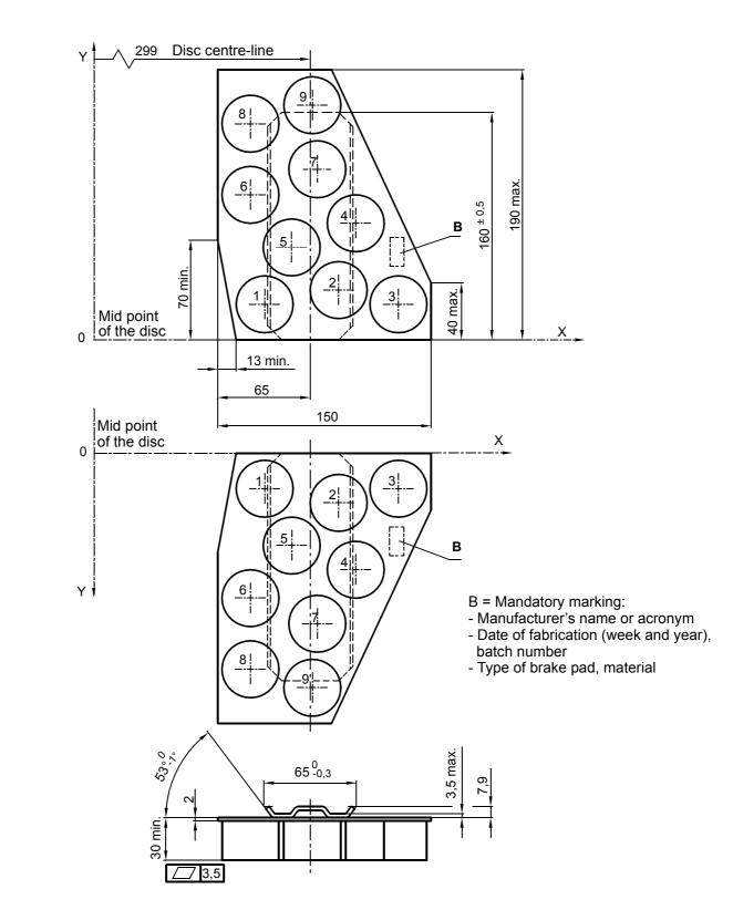
**NB :** The sum of the rubbing surfaces in this case is the sum of the surfaces of the nine circular shaped rubbing elements of a pad half.
