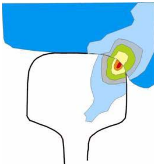
Fig. 9 - Head-checking emergence zone
