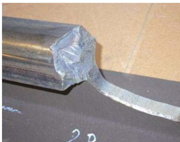
Fig. 12 - Example of a breakage under a squat
