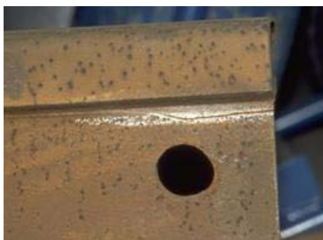
Fig. 5 - Typical example of a horizontal crack on a rail end
