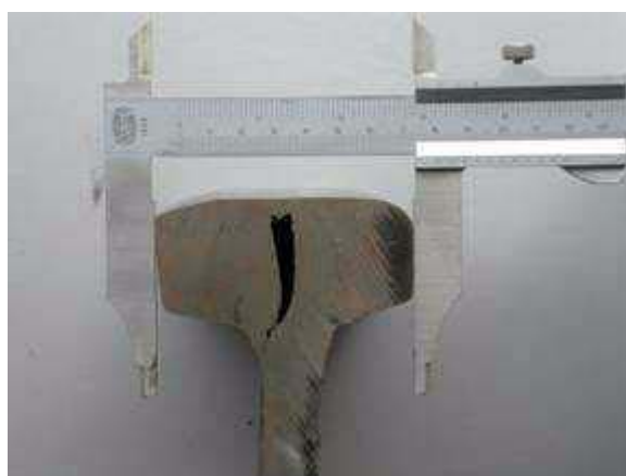
Fig. 6 - Typical example of a longitudinal vertical crack at stage 2. At this stage, the crack can be detected easily by ultrasound.
