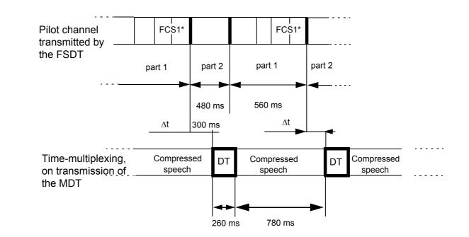
**NB** :  $\Delta t$  = time interval between radio reception of the last bit of the FCS1\* of an initial part of a message on the pilot channel and beginning of a period allocated to radio transmission of traffic messages. This time must be equal to 300 ± 5 ms to take into account the transmission times within the mobile unit.
