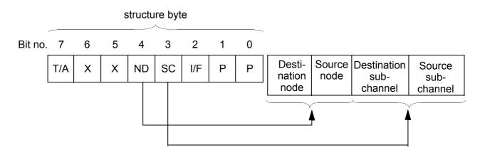
The first structure byte specifies the nature of the information which follows it. This byte has the following composition:
