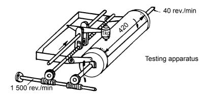
At each revolution of the cylinder, the test-piece is raised from the abrasive surface for a certain period suddenly but without jerking, and then brought into contact again with the latter. The lifting movement shall be regulated so that the test-piece is subjected to wear by the abrasive surface over a length of 400 mm for each revolution of the cylinder.
