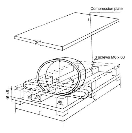
After 10 minutes, the flattening pressure is removed, and the external vertical diameter  $D_1$  is again measured and recorded after a further period of 1 minute.
