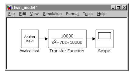
You next task to enter parameters for the Analog Input block. See "Analog Input Block" on page 4-12.
