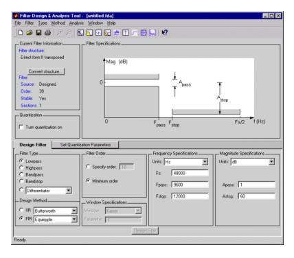
To start the tool, type fdatool at the MATLAB command line.
