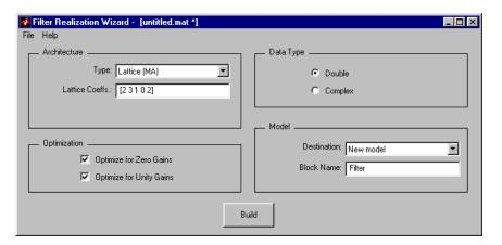
When you click the GUI's **Build** button with the particular settings shown above, the wizard constructs the specified moving average (MA) lattice architecture as a subsystem within a new model window.
