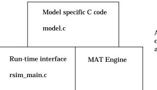
An RSim simulation consists of models as shown.
